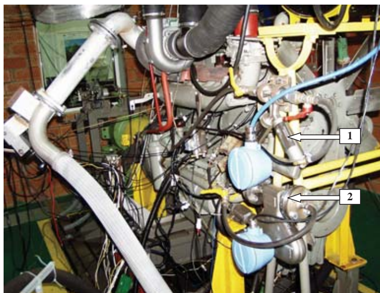
Fig. 3. View of test stand with flowmetering system of fuel consumption measurement: 1 - flowmeter to measure of fuel flow rate to the engine, 2 - flowmeter to measure of fuel flow rate from the engine
